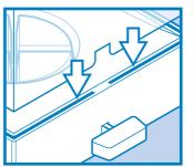
Make sure that the central notch is aligned on each side.
