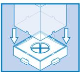
O4 Slot the walls into the base, as shown.
