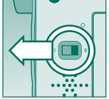
Carefully lift the bog and move the ON/OFF switch to the 'ON' position.
