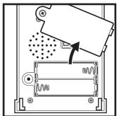
**B** Remove the battery compartment cover.
