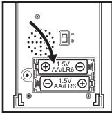
C Insert 2 AA/LR6 batteries with the polarity as shown. Replace the battery compartment cover and tighten the screw gently.
