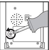
A Turn the unit over. Using a cross head screwdriver, turn the battery compartment screw anti-clockwise.
